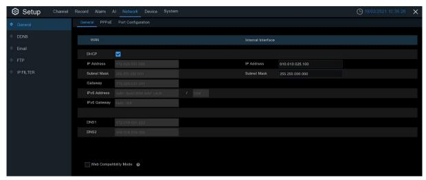
If you connect to a router allows to use DHCP, please check the **DHCP** box. The router will assign automatically all the network parameters for your NVR. Unless the network is manually addressed below parameters:
