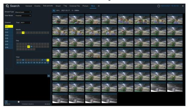
Choose the video stream type, channel, date and hour. The system will display 60 thumbnail images of each minute on the screen. Click on any one of the thumbnail images, the video will be played on the left bottom corner.
