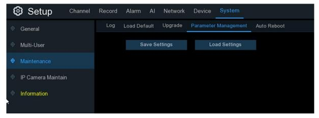
**Save Settings**: Click to save the NVR current system settings to the USB device. You will be required to input the Admin password to authenticate.
