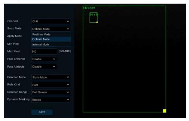
**Apply Mode:** Set the face detection angle, including "Frontal View", "Multi Angle" and "Customize" mode.
