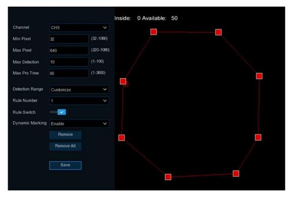
Min Pixel: Set the minimum detection pixel box. The people can be recognized only when he/she is larger than the pixel box.
