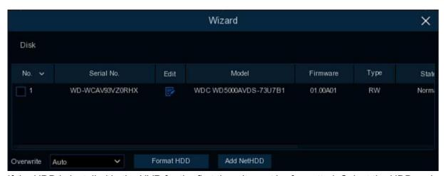
If the HDD is installed in the NVR for the first time, it must be formatted. Select the HDD and then click **Format HDD** button to format the HDD.
