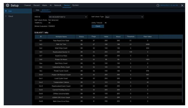
Whole Evaluation not passed, continue to use the disk: If for some reason the hard drive has developed a fault (such as one or more bad sectors), you can instruct your NVR to continue saving to the drive.
