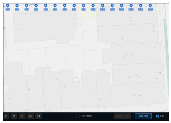
3. Click ① icon to select one face image from local storage or external USB storage. Select date & time, group(s), channel(s), set the similarity rate, and then click Search button. The system will display the result on the e-map. If the person was captured by multiple cameras, the system will display his/her moving track on the map.
