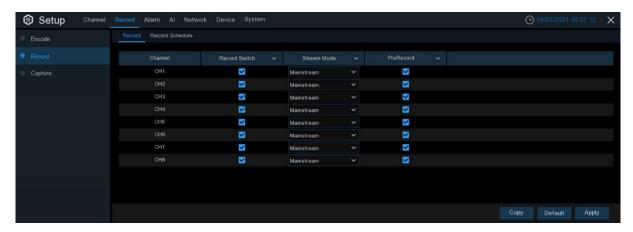
**Record Switch**: Check to enable the recording in this channel.
