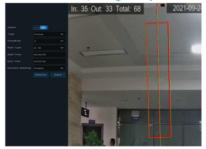
Switch: Activate or inactivate the detection.
