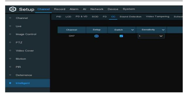
Switch: Check the box to enable CC function.
