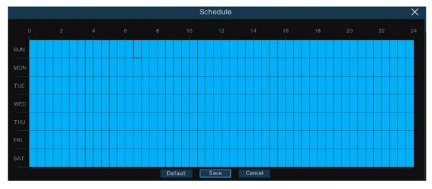
When the time slot is marked light blue, this indicates the channel triggers deterrence alarm for that time slot.
