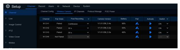
You can configure the connection of compatible wireless IP cameras in this page which is disappeared if none of the channels is set to Wireless mode in the Channel Config page.
