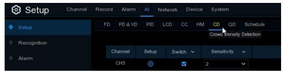
Switch: Check the box to enable the CD function.
