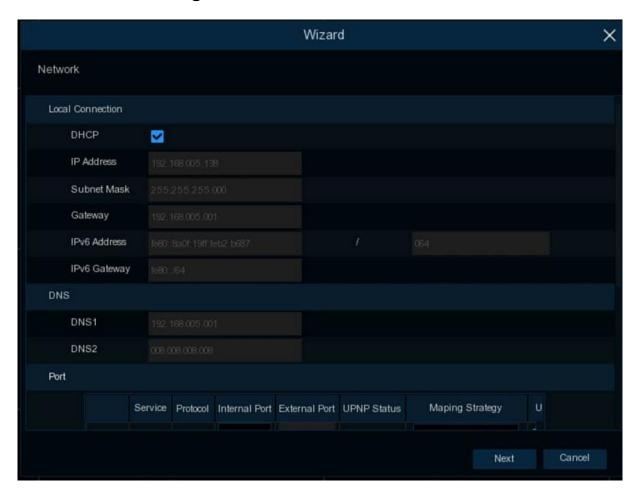
If you connect to a router allows to use DHCP, please check the **DHCP** box. The router will assign automatically all the network parameters for your NVR. Unless the network is manually addressed below parameters:
