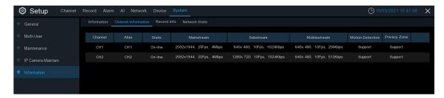
View channel information for each connected camera such as alias, mainstream and substream recording specifications, motion detection status & privacy zone.
