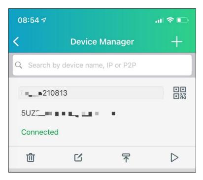
6. If your mobile is connecting to the Wi-Fi which is in the same LAN with your NVR, you can choose to add the NVR by using Online Search. Touch on the device in the search result list, and then input the port, use name, password to add.
