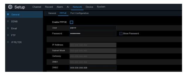
This is an advanced protocol that allows the NVR to connect to the network more directly via DSL modem.
