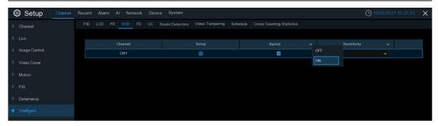
Switch: Check the box to enable SOD function.
