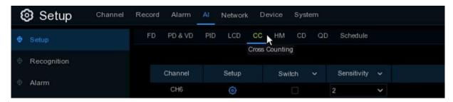
Switch: Check the box to enable the function.
