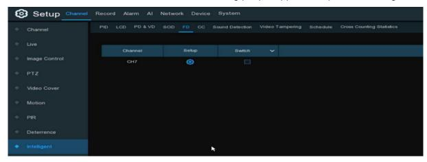
Switch: Check the box to enable FD function.
