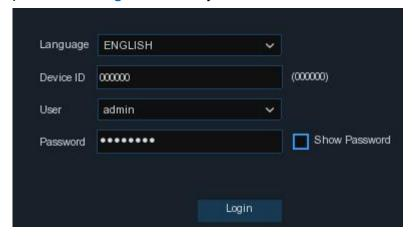
**NOTE:** If you forget your password, you will be unable to login the system, please contact your reseller to reset the password. If your NVR has a reset button in the rear panel, press and hold 3 seconds to reset password.
