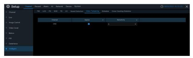
Video Tampering detects the occlusion of the live view screen, and some certain actions can be taken when the alarm is triggered.
