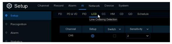
Switch: Check the box to enable the LCD function.
