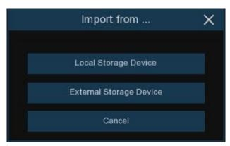
Click Local Storage Device to import face images which were captured and saved in the NVR local HDD storage.
