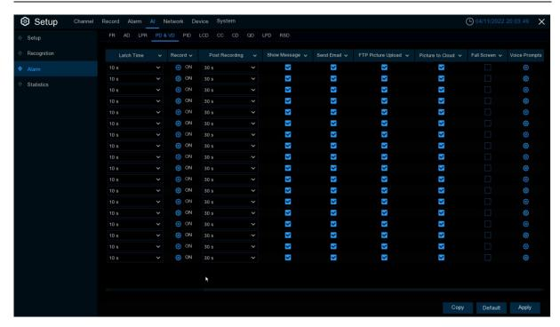
Configure the pedestrian and vehicle alarm function
