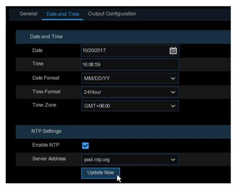
Check to enable the NTP, and select a Server Address, click Update Now to manually sync the date & time.
