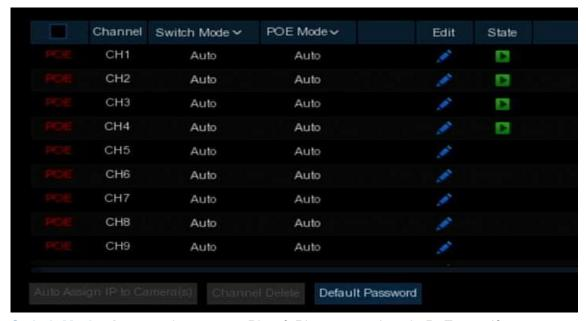
**Switch Mode: Auto** mode supports Plug & Play connection via PoE port. If you want to add camera(s) manually then change the mode to **Manual**.
