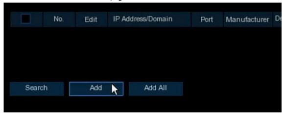
2. Input the IP address or domain name, port, protocol, user name & password of the IP camera. Click **Add** button to add the camera.
