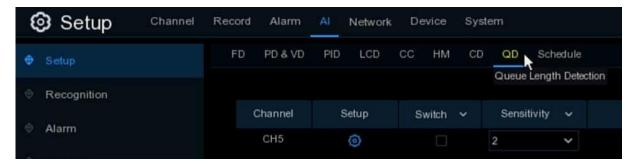
Switch: Check the box to enable the QD function.
