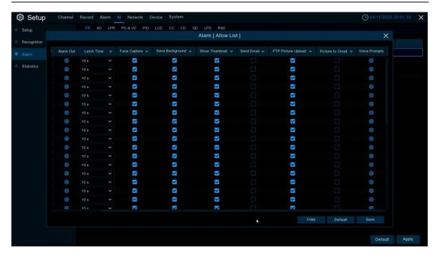
**Alarm Out:** optional function. If your DVR supports connecting to an external alert device, you can set up an external alert device.
