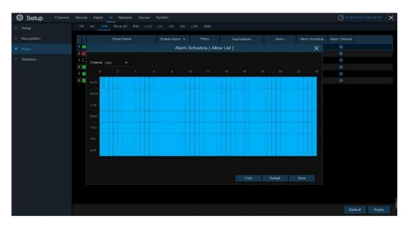
Check the time period that you want to alarm, Click **Apply** to save. Click **Copy** to copy the current channel parameters to other channels.
