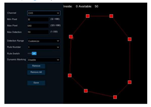
Min Pixel: Set the minimum detection pixel box. The people can be recognized only when he/she is larger than the pixel box.
