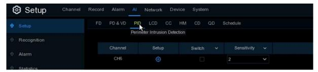
**Switch:** To enable or disable the Perimeter Intrusion Detection.
